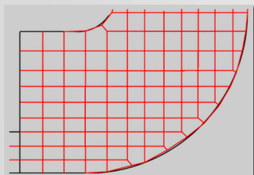
TAG mesh for an accurate representation of the casting geometry.
