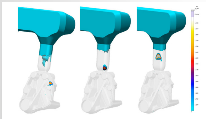
An accurate description of the flow front shows entrapped air in the casting system.
